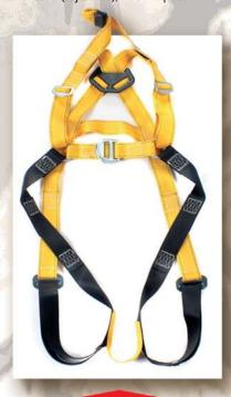
**SEH5** - WORKER RESCUE HARNESS full-body harness with front and rear attachment for fall-arrest and extra rescue strap for confined space ascent, descent and rescue (in cooperation with tripod/winch as mentioned on page 13).
